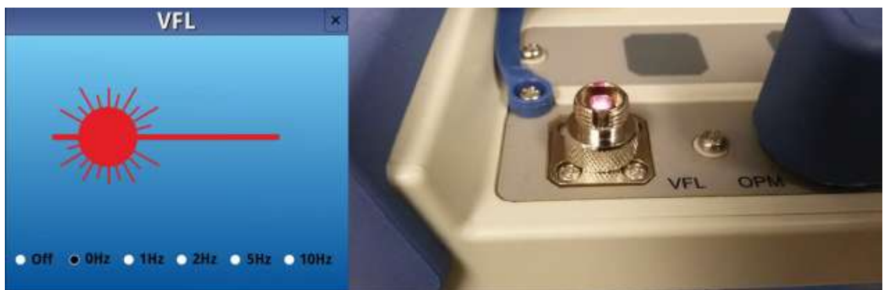
Pictured: Visual Fault Locator (VFL) beam illuminates bends, splices, and faults in optical fibers.
